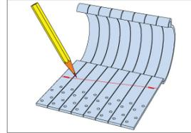
Mark the hangers for the gutter incline. 1/16 to 1/8" per 3ft.
